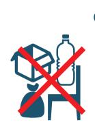
Use only dry **natural wood** that has not been treated, or EN-Plus certified pellets. Never burn waste (not even paper, cardboard, coloured magazines, plastic, styrofoam, treated wood, furniture) as they release toxic substances (such as formaldheyde and dioxin). Use the appropriate firelighter cubes in order to light the systems.
